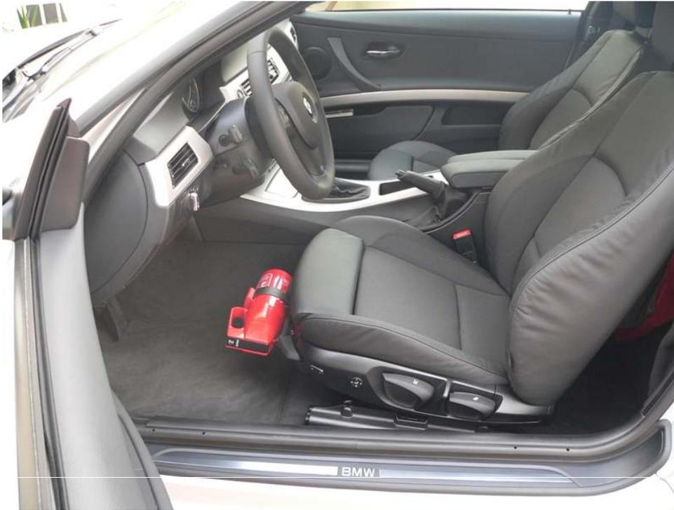
OEM BMW fire extinguisher installed under driver's seat in an E92 model.
