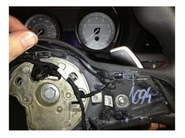
$\circ$  The blue connector on the left slides under a tab on the left multifunction button assembly
