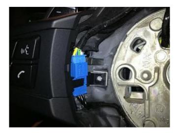
• Partially line up the airbag pins with their holes
