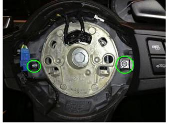
• Pull the multifunction buttons and their surrounding trim out of the steering wheel. It seems easiest to start with the lower inside corner. They're held in by the two tabs you see sticking out
