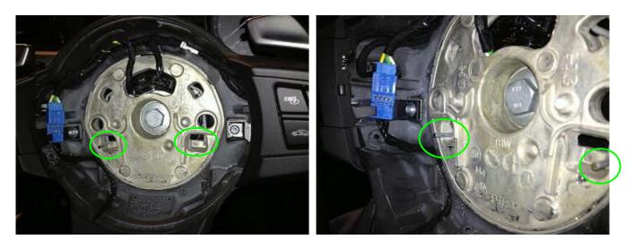
• Disconnect the wire harness and set the airbag off to the side. Make a note of how the posts coming out of the back of the airbag line up with the holes in the steering wheel frame (arrow in blue)
