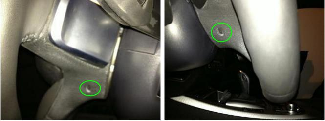
• Insert the long thin screwdriver into each side, nearly vertically, and compress the spring to release each side of the airbag
