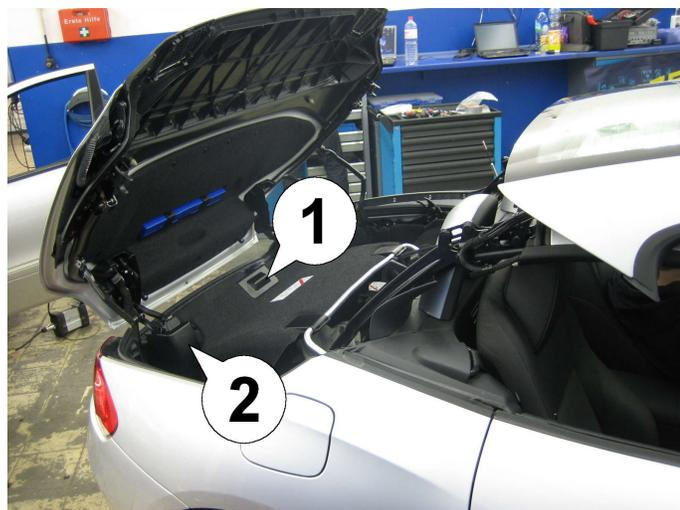
1. Turn ignition on and open convertible top to the shown position (service position), then stop. **Now turn ignition off and pull key before continuing!** From the right side, reach into the trunk and lift the luggage divider (1) into the upper position. Then remove plastic cover (2) by pulling toward the front of the car. It is only held in place by three spring locks.
