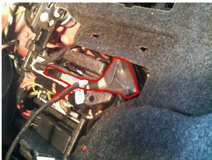
9. The best way to stow the bulky harness and connectors in the tight space is shown here. This way the lid(s) can be reinstalled without problems.
