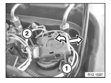
Unlock plug catch (1) of ignition coil (2) and disconnect plug.
