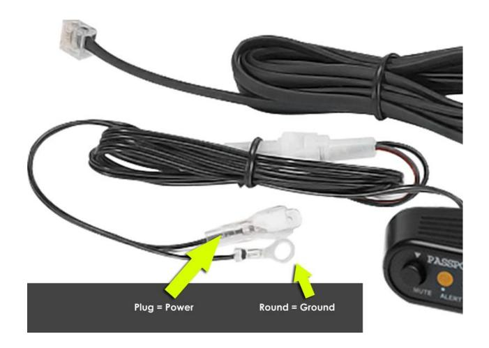
10. Using the wire strippers, cut the end of the power line, just before the plastic sheathing. Again, this is the wire that has a flat plug connector.
