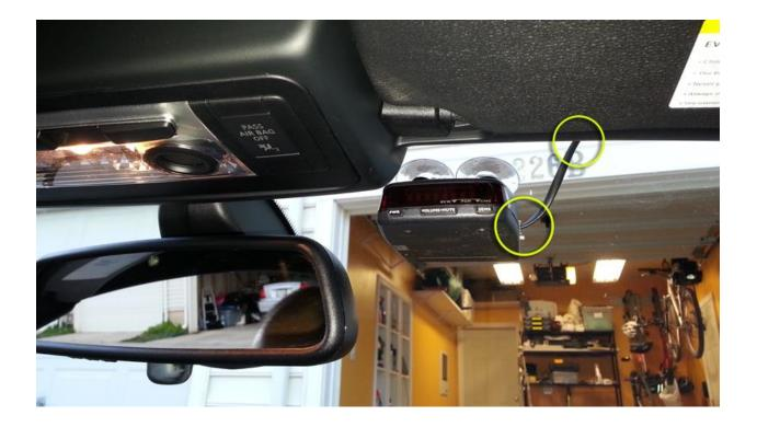
19. You can tuck the wire coming out of the radar detector into the forward-edge of the trim where it meets the windshield. Follow this seam down the forward edge of the a-pillar. Make sure that as you tuck the wire into the seam that you keep the cable flat (I had to continuously fight the cable to keep it from being twisted).
