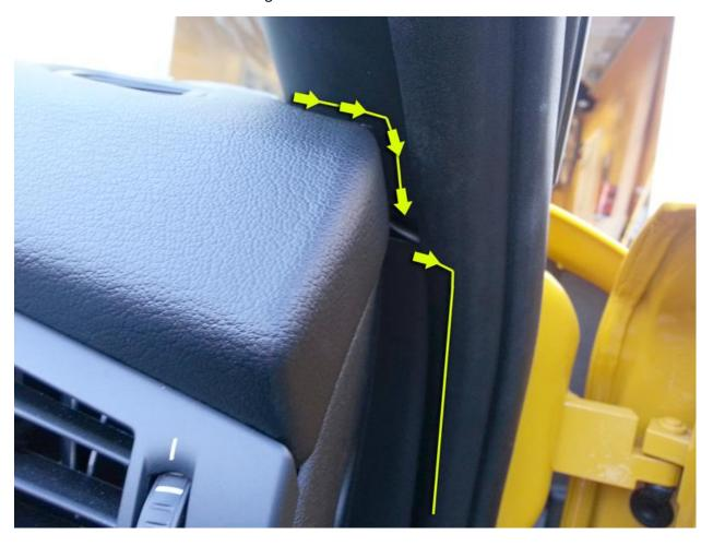
22. Run the wire down the inside of the weather stripping until you reach the 2<sup>nd</sup> horizontal gap in the trim at beginning of the footwell. Bring the cable back through this gap and along the upper right corner of the footwell.
