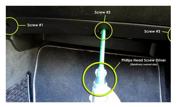
2. Carefully remove the panel (that was secured by the 3 screws that were just removed). Be sure to apply pressure towards the right on the left-most corner of the panel as you pull it down to ensure that the corner of the panel does not scratch the leather where it meets the center console. There should be enough flex in the panel to bend it as you pull it down to avoid scratching/scuffing.
