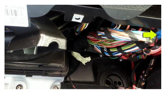
6. Twist the Fuse Panel Release tab (Shiny Fastener) counter-clockwise. Using your hand / fingers continue to unscrew this tab until the fuse box panel drops down / is released.
