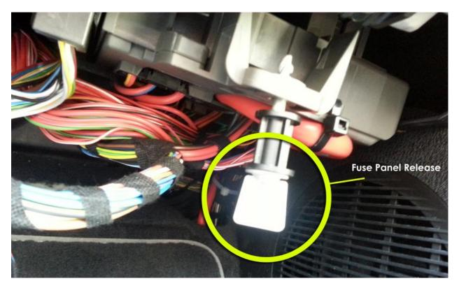
7. Slowly pull the fuse box panel down, sliding it towards you as you go. The fuse box panel is connected to a green rail, allowing it to slide.
