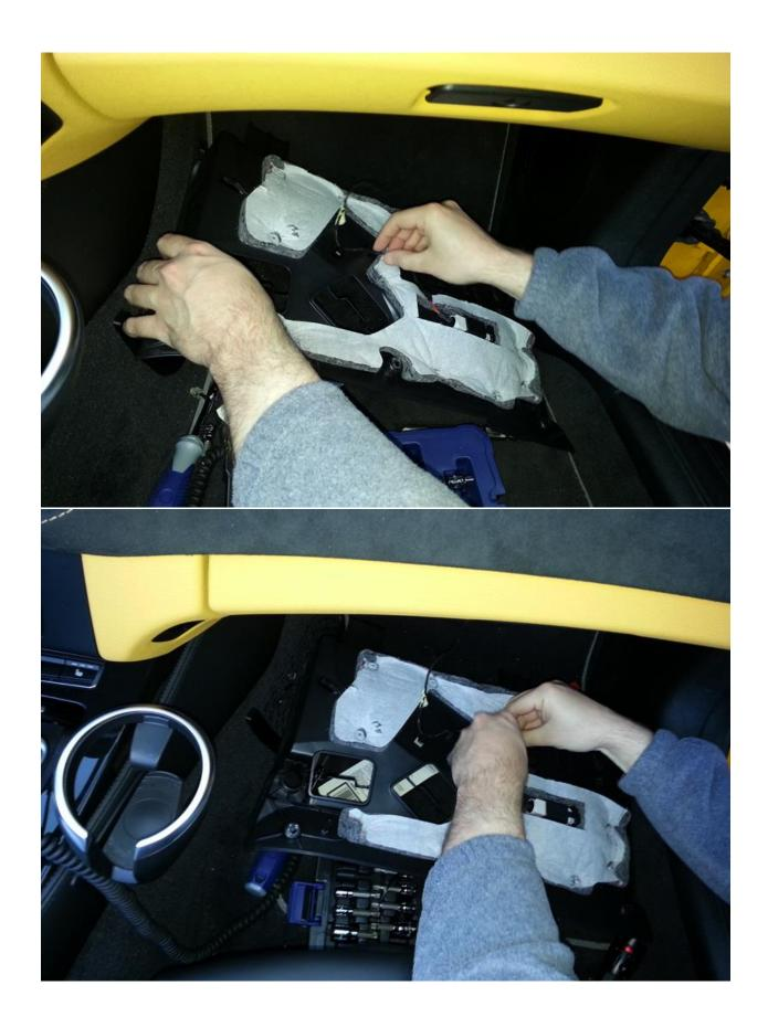
31. Once the power cable is reconnected, re-install the body panel into its original position. Make sure to keep a hand / eye on the left upper-most corner of it to ensure that you do not scuff the leather on the center console. It took a few tries before I successfully got the panel seated towards the front of the car and the screw holes were correctly lined up.
