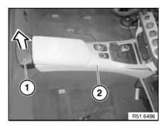
Remove rear cover (1) from centre console (2) towards top. Disconnect plug connection underneath.
