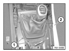
Unclip cable routing (1) from centre console (2).
