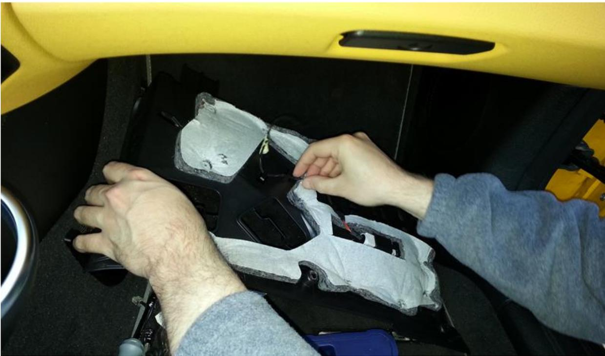
4. Once the panel is resting on the floor of the car, disconnect the cable / plug that powers the "mood lights" in the footwell. With this cable disconnected, you can now remove the panel in an effort to get it out of the way.
