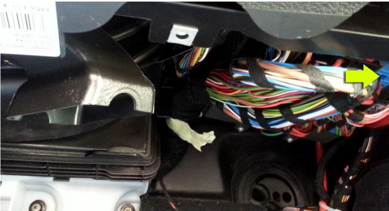
6. Twist the Fuse Panel Release tab (Shiny Fastener) counter-clockwise. Using your hand / fingers continue to unscrew this tab until the fuse box panel drops down / is released.
