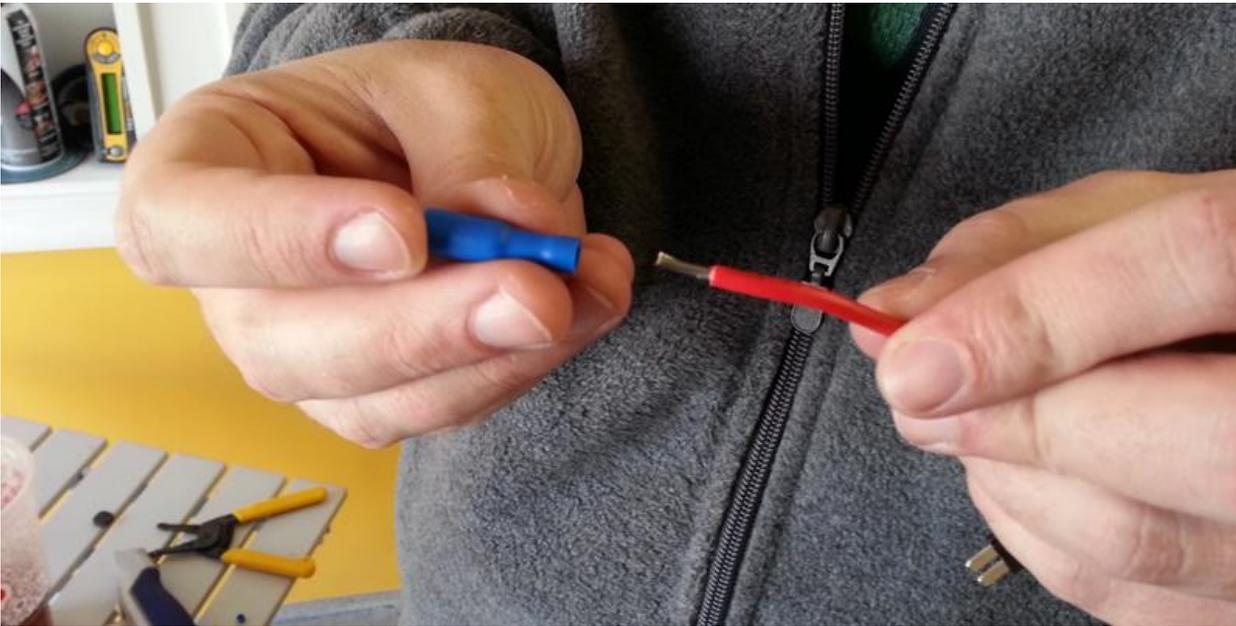
15. Connect the male and female ends of the 16-14 Gauge (5/32") Bullet Connectors.
