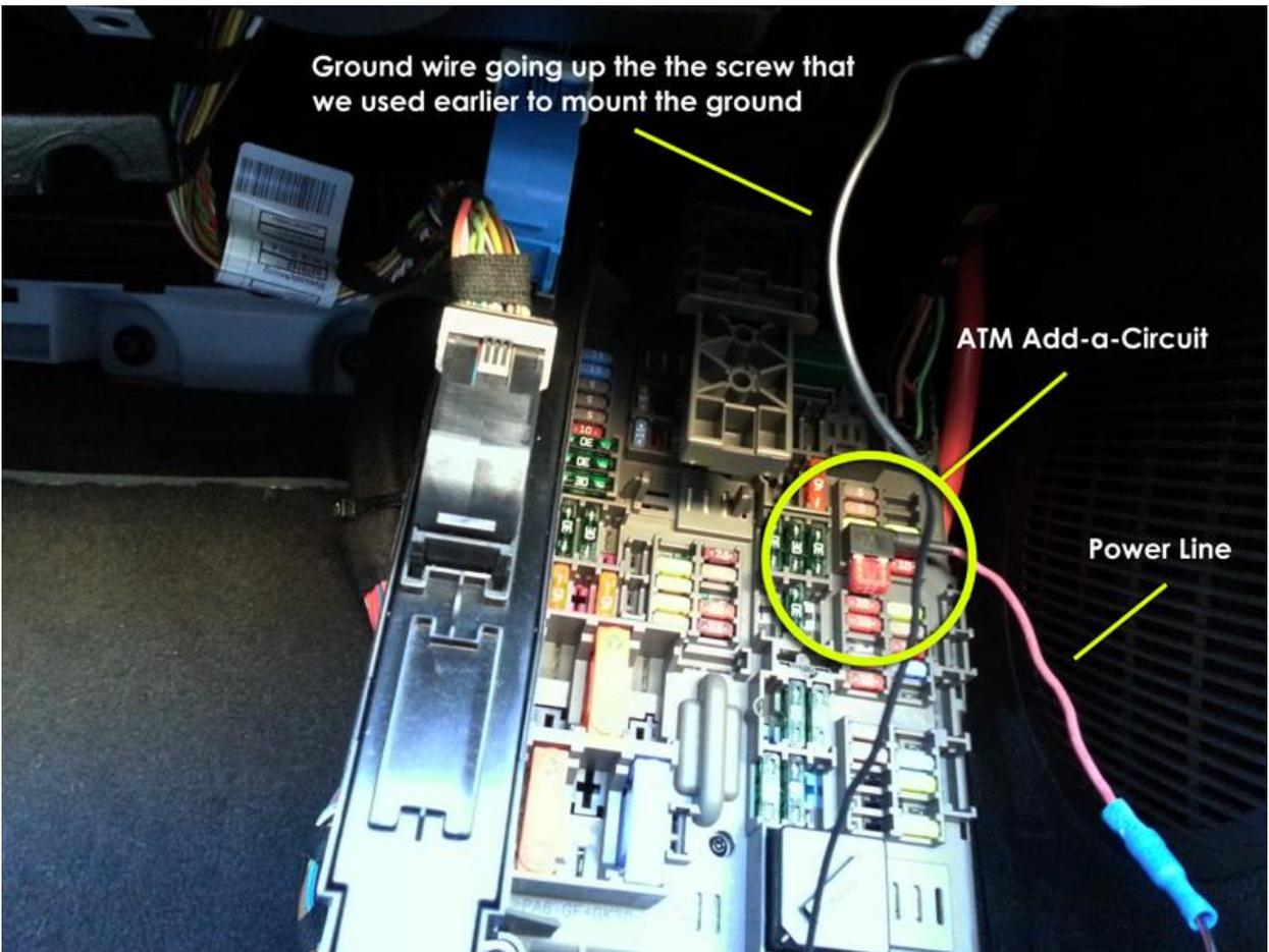
26. Once you have the power and ground connected, run through a test of the radar detector's functionality. The car has some strange power states, so for "being certain's sake" I would go from all the way off / nav screen retracted / no lights of any kind on to all the way on / engine started.
