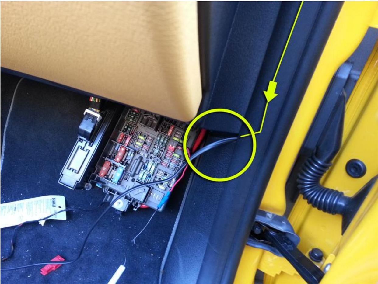
23. Next we will mount the ground wire from the radar Direct-wire cable. Using a T-15 Torx bit, remove the screw (shown below) found near the place that the “Shiny Fastener” was connected to the trim on the underside of the glove box area.
