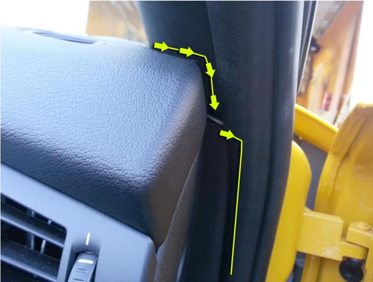
22. Run the wire down the inside of the weather stripping until you reach the 2<sup>nd</sup> horizontal gap in the trim at beginning of the footwell. Bring the cable back through this gap and along the upper right corner of the footwell.
