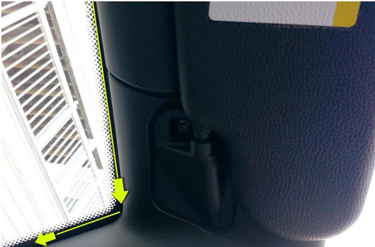
20. When you come to the base of the a-pillar, there is a somewhat sharp turn that you'll have to make. It helped me to run the cable an inch or so to the left along the base of the windshield prior to coming back towards the pillar.
