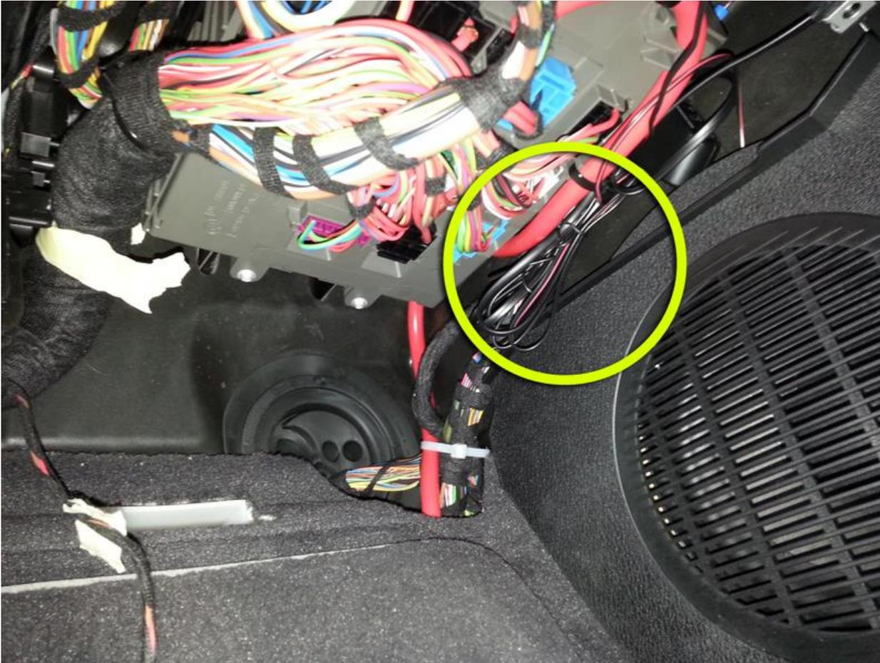
28. I took the picture (above) after I had already raised the fuse box panel back up into its secured position. Make sure that when you are raising the fuse box panel to slide it back up it's rail and be mindful of the bundle of cable that you've place to the right of it. Make sure not to pinch any of the cables. Use the "Shiny Fastener" to secure the fuse box, twisting it clock-wise until its tight.
