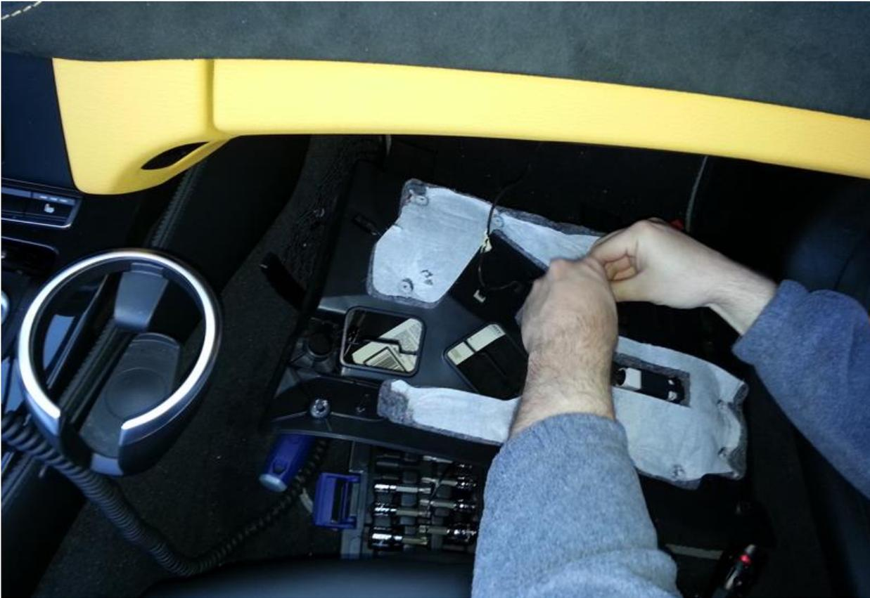
31. Once the power cable is reconnected, re-install the body panel into its original position. Make sure to keep a hand / eye on the left upper-most corner of it to ensure that you do not scuff the leather on the center console. It took a few tries before I successfully got the panel seated towards the front of the car and the screw holes were correctly lined up.
