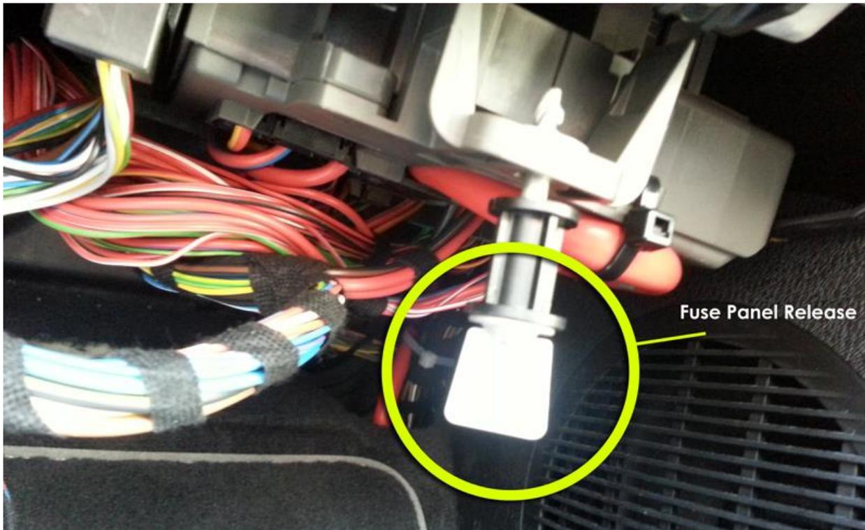
7. Slowly pull the fuse box panel down, sliding it towards you as you go. The fuse box panel is connected to a green rail, allowing it to slide.
