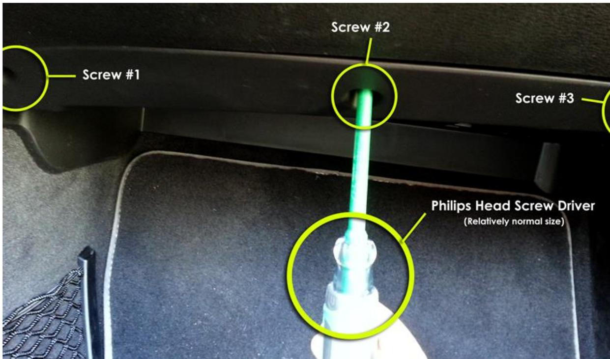
2. Carefully remove the panel (that was secured by the 3 screws that were just removed). Be sure to apply pressure towards the right on the left-most corner of the panel as you pull it down to ensure that the corner of the panel does not scratch the leather where it meets the center console. There should be enough flex in the panel to bend it as you pull it down to avoid scratching/scuffing.
