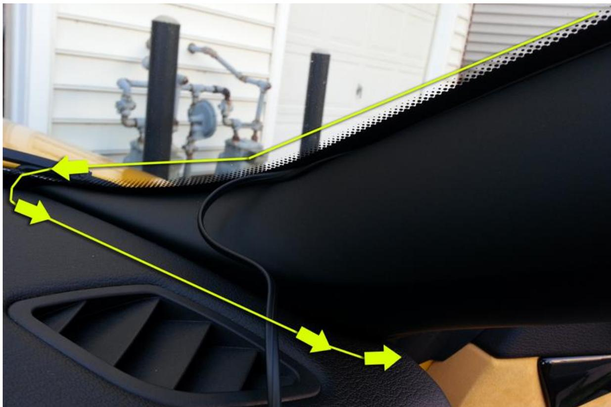
21. Tuck the cable into the seam along the base of the a-pillar. This seam can be a bit tight. Having a credit card or something similar to push the cable into the seam may be helpful. Keep tucking the wire in along this piece of trim downward until you reach the small horizontal gap shown in the picture below. Bring the cable from the seam through this gap to the weather seal running down the car's frame. Be sure to tuck the cable (without twisting) as far under the weather seal that it can go.
