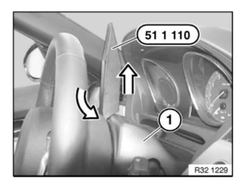
Move steering column into "lower" and "extended" position.
