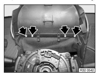
Tilt steering column trim forwards. Unclip gap cover from steering column trim.
