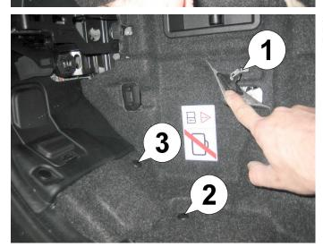
3. Now pull up on the bottom of the carpeted piece to reveal two more spring locks (1). Remove the plastic plugs (2) and (3) to remove the whole carpeted piece.
