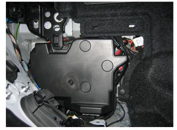
4. Remove additional plugs (1) and (2) that hold the plastic cover in place. One (see arrow) is hidden right behind the trunk lid hinge. Remove the whole plastic piece.
