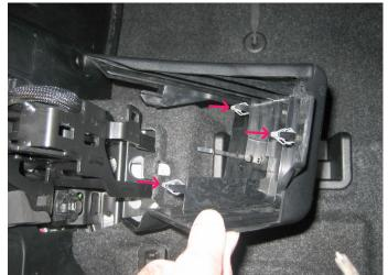
2. The spring locking mechanisms are marked here with arrows.
