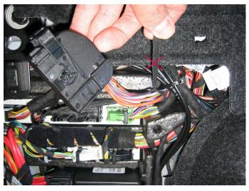
7. Remove the black plug from the top controller and replace it with the one from the SmartTOP wiring harness. Make sure the lever locks into place. Since the introduction of the plug and play wiring harness, the cloth tape does NOT have to be removed (as seen here) any more!
