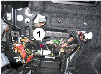
6. The convertible top controller is white and easily distinguished by a bright green and a long black connector. Push down on the locking tab (1) while moving the lever to the left (arrow) to remove the black connector from the controller.
