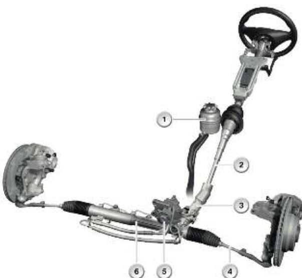
Hydraulic power steering (typical installation configuration)
