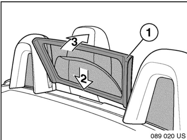
1. Remove the roll over covers from the roll over bar per RA 514 30 30.
